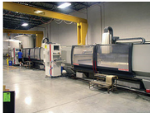
The Millbury facility also operates two Intermac Master Stone CNC stoneworking centers, and a third one is in operation in Wallingford.
