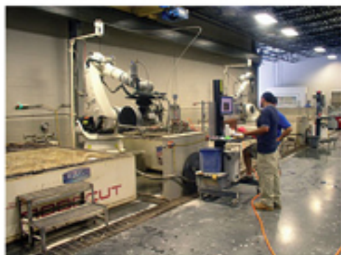
The Millbury facilities added two RoboCuts from USG Robotics. The machines offer 6-axis waterjet and saw cutting.
