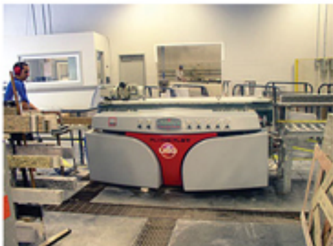
A Flying Flat edging machine from Sassomeccanica is used for processing backsplashes.
