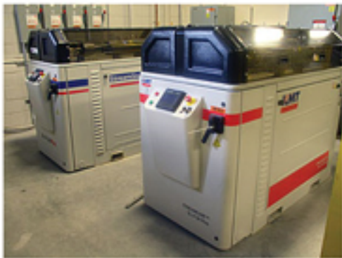
Each RoboCut is equipped with a 50-horsepower waterjet pump and nozzle from KMT of Baxter Springs, KS, for precise cutting.
